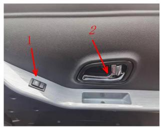
1. This is the window switch. It should be noted that when the glass is completely raised or lowered, please immediately release the button. Otherwise, it is easy to damage the lifting motor.
