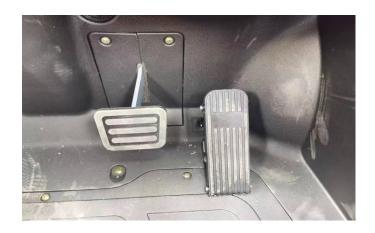
On the left is the brake pedal, and on the right is the accelerator pedal
